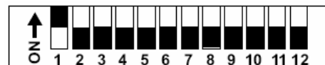
Figure 16: Dip Switches should be in “UP” position for each IR Sensor used
